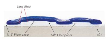
Figure 4: Cross-sectional view of kilnformed glass, fired at 1420°F (~770°C).
